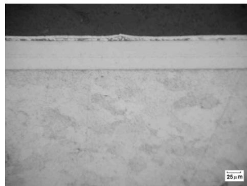
Fig. 8. Micrograph of a nc-Ti 2 N/nc-TiN nanocomposite coating with a thickness of 52 μm deposited on plain carbon steel.
