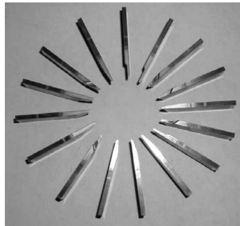
Fig. 10. Turning cutters coated with nc-Ti 2 N/nc-TiN nanocomposite coating.
